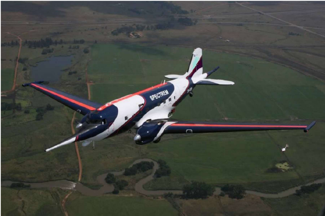
Figure 1: The specialised Spectrem aircraft that will carry out the SpectremPlus™ airborne electromagnetic (AEM) survey over the Zeb Nickel Project area.
