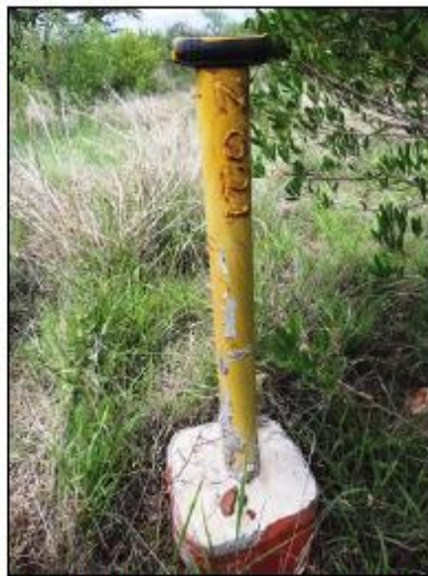
Collar stand pipe for drill hole Z021.
